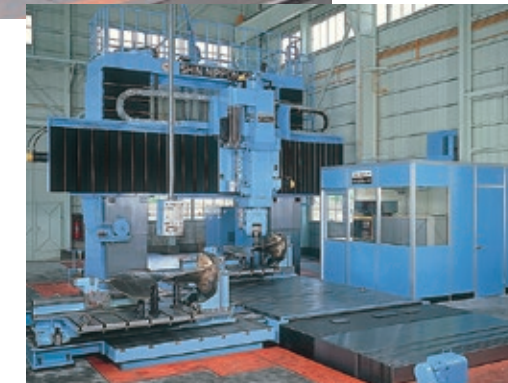
6軸同時5軸NC翼面加工機 6 Axes with simultaneous 5-axes control NC blade milling machine
